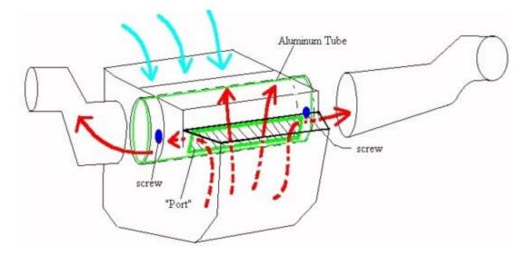
There is nothing between the two oval-shaped outlets on the heater box, so i went to Home Depot's HVAC duct area and picked up a 3" diameter aluminum heater duct for £2 or 3. This is a rolled sheet that is not joined to form a tube, but rather has a seam that can be snapped closed.
